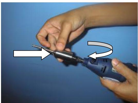
**Put the shaft tube onto the axle and screw clockwise onto the housing!**
