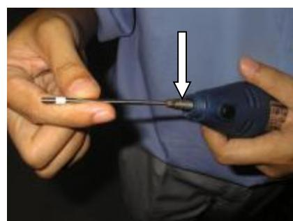
**Remove collette and insert axle of the shaft into its place!**
