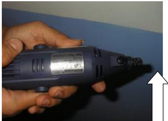
**Hold HOMOGENIZER drive open the collete and press the black button to lock it and unscrew the collete**
