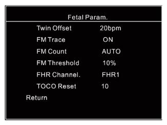
Twin Offset: In twins state, to avoid FHR2 curve coinciding with FHR1 curve, lower the position of FHR2 curve for several unit points, which are the curve separating values; available options are 0, 20, 30; 0 indicates no separation. Unit: bpm.
