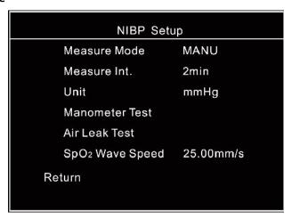
Measure Mode: Blood pressure measurement mode: "Auto" and "Manual" are available.
