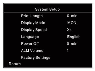
Print Length: Set the printing duration (up to 60min); when the print time is up, printing stops. 0 indicates that the function is invalid.
