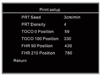
PRT Speed: Adjust the printing speed; available options are 1cm/min, 2cm/min, and 3cm/min.
